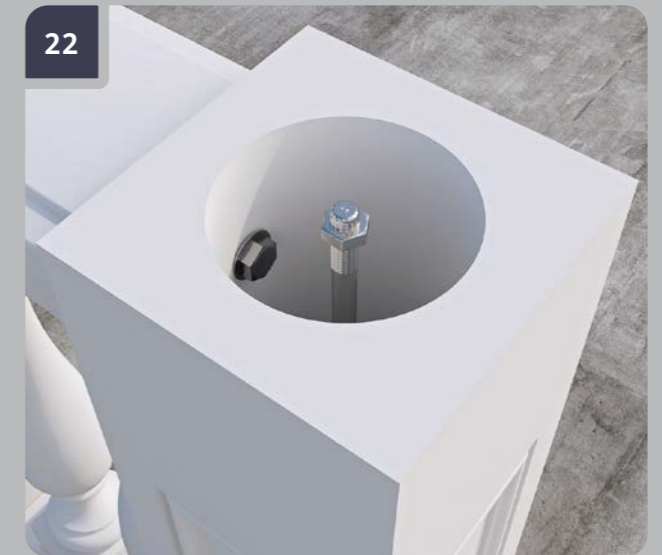
22 Fasten the newel to the handrail with a bolt.
